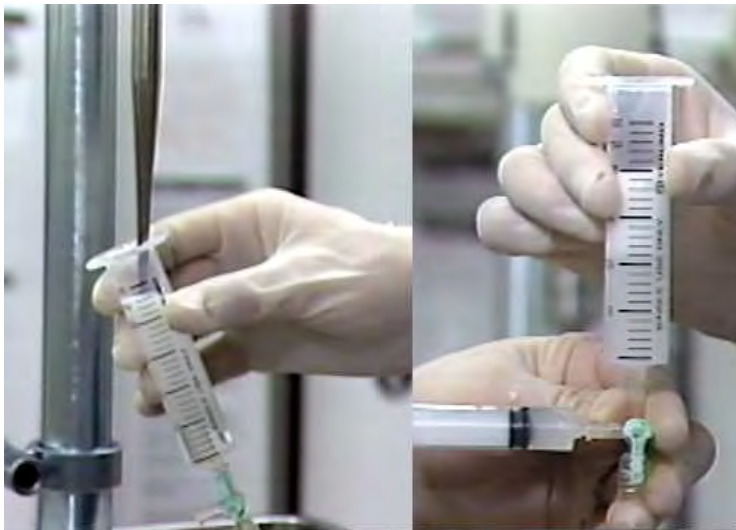
Fig. 1. Sonification of contrast medium to make microbubbles for MCE
