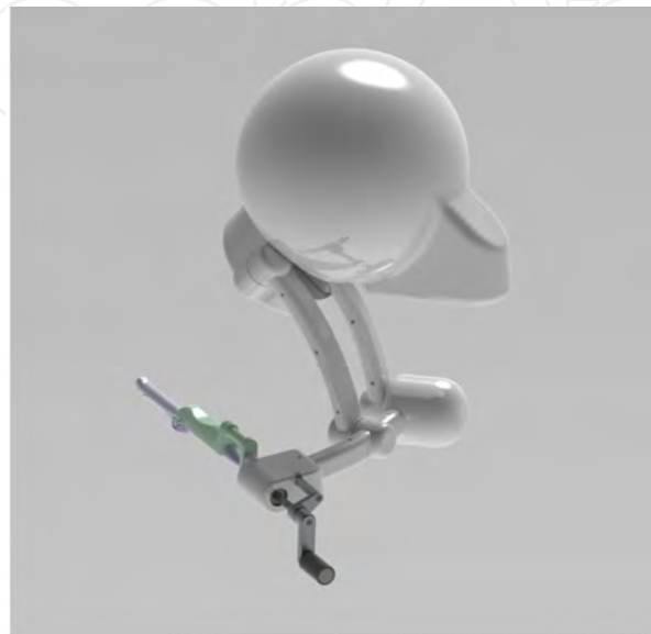
Figure 8. A schematic diagram of the mechanical tracker, which supports the TRUS transducer and attached cradle. This configuration constrains the TRUS probe motion to three degrees-of-freedom and one degree of translation along the axis of the probe. The system is mounted at the base of a stabilizer while the linkage allows the TRUS transducer to be manually manipulated about a remote center of motion (RCM), which is at the center of the ultrasound transducer tip.
