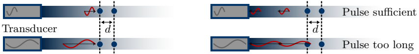
Figure 11.6: Axial resolution: illustration of dependence on wave frequency f . Left and right shows two different timesteps, where d denotes the distance between two structures (blue dots). The high frequency (top) wave allows for distinguishing between the two structures, as clearly separated echoes are sent back to the sender. Using the low frequency wave, the echoes cannot be separated (echoes are merged).
