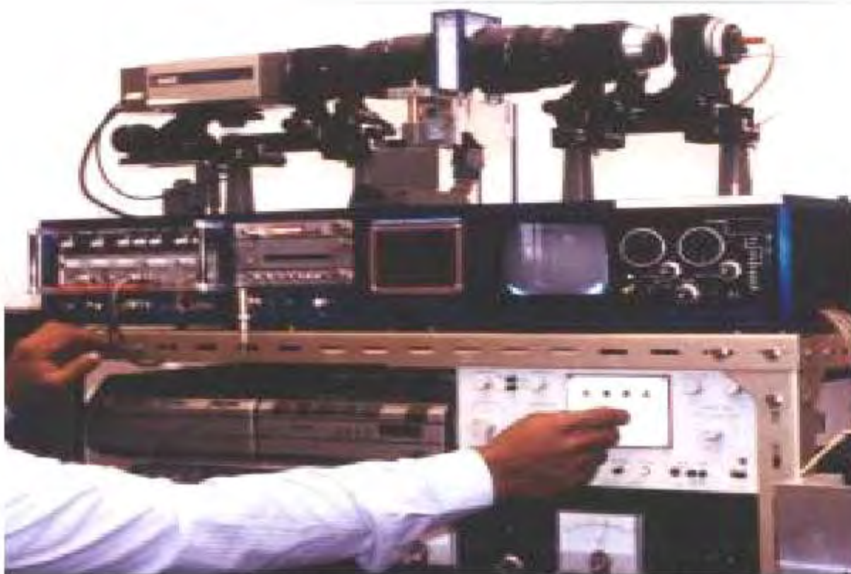
Figure 9. The active acoustooptical imaging system (1 st prototype)
